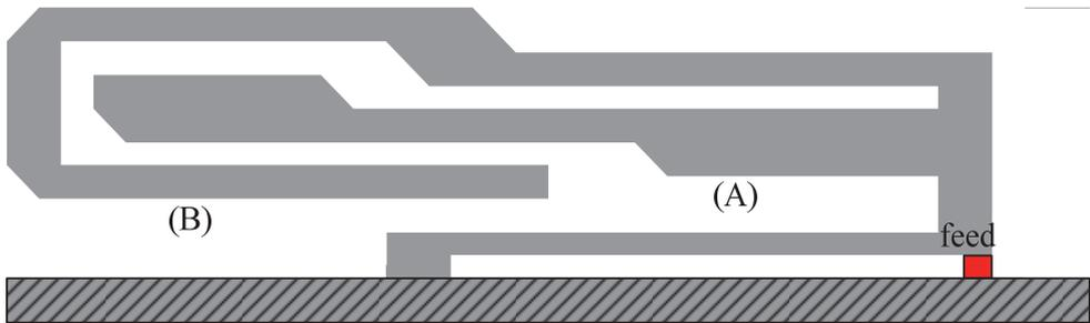
Fig. 5. A dual band inverted-F main resonator.
