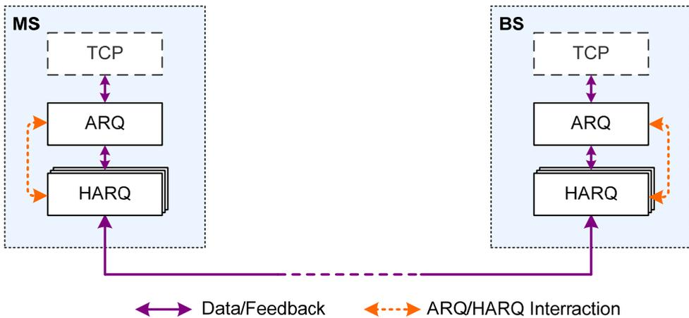
Fig. 3. Principle of ARQ and HARQ cooperation
